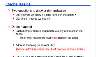
Have a tag associated with each cache block that contains the address information (the upper portion of the address) required to identify the block (to answer Q1)
