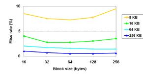
Miss rate goes up if the block size becomes a significant fraction of the cache size because the number of blocks that can be held in the same size cache is smaller (increasing capacity misses)
