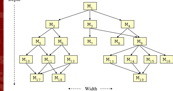
M<sub>9</sub>: Fan-in = 2, fan-out = 4
