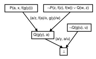
Note that the unifying substitutions are applied to entire clauses, and not just to the atoms to be matched. The tail-recursive call graph for the processing of  $\psi_1$  and  $\psi_2$  is shown below. Only the most significant procedure calls are shown:
