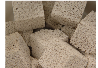
Porous ceramic with interconnected pores that vary in size from 5–500 μm. (Source: Wikimedia commons).
