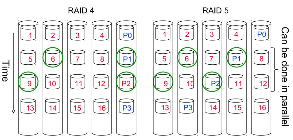
By distributing parity blocks to all disks, some small writes can be performed in parallel
