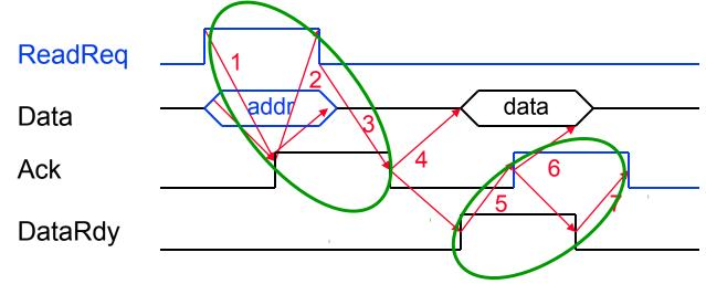
I/O device signals a request by raising ReadReq and putting the addr on the data lines
