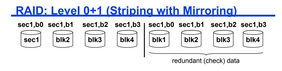
Combines the best of RAID 0 and RAID 1, data is striped across four disks and mirrored to four disks
