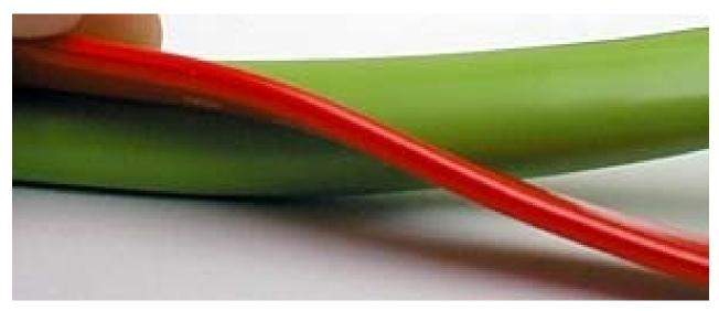
Serial ATA cables (red) are much thinner than parallel ATA cables (green)
