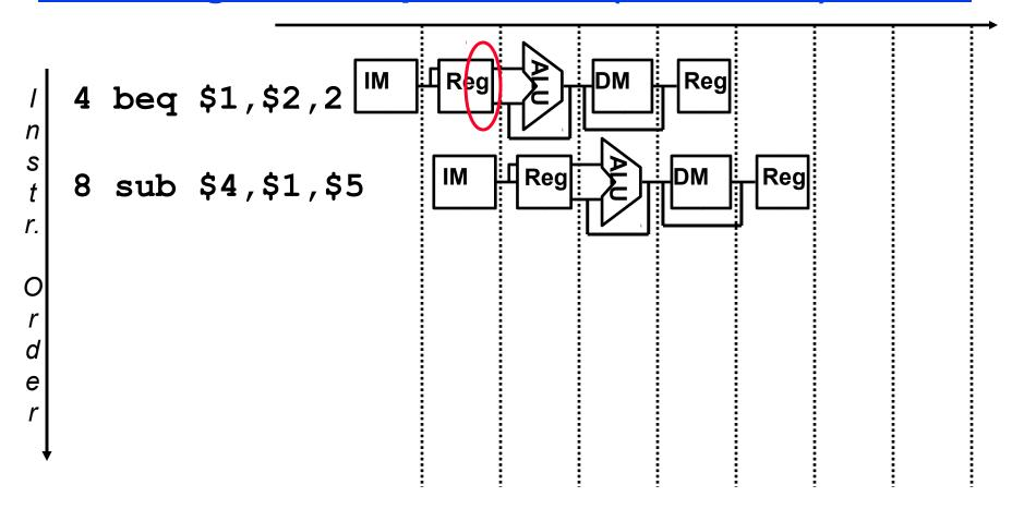
To flush the IF stage instruction, assert IF.Flush to zero the instruction field of the IF/ID pipeline register (transforming it into a noop)
