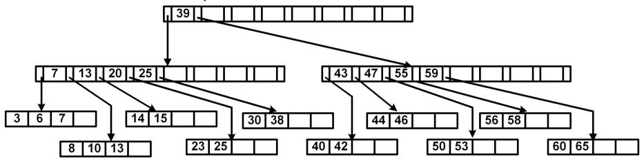
Continuation of the deletion example; deletion of 38 with a reduction in depth:
