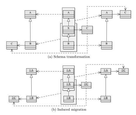
Fig. 15: Moving the origin of an association upwards the inheritance hierarchy
